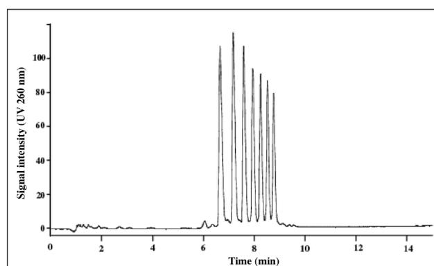
**Figure 8.** Column, poly(3-diethylamino-2-hydroxypropylmethacrylate-co-divinylbenzene), monolithic, 80 mm  $\times$  0.2 mm i.d. Mobile phase A: 20 mM  $\text{KH}_2\text{PO}_4$ , 20% ACN, pH 7.0; B: 20 mM  $\text{KH}_2\text{PO}_4$ , 20% ACN 1 M NaCl in A; gradient, 25–55% B in 2 min, 55–100% B in 7 min; flow-rate, 2.3  $\mu\text{L}/\text{min}$ ; room temperature; detection, UV, 260 nm; sample,  $d(\rho\text{T})_{12-18}$ . Reproduced from Reference 68 with permission.
