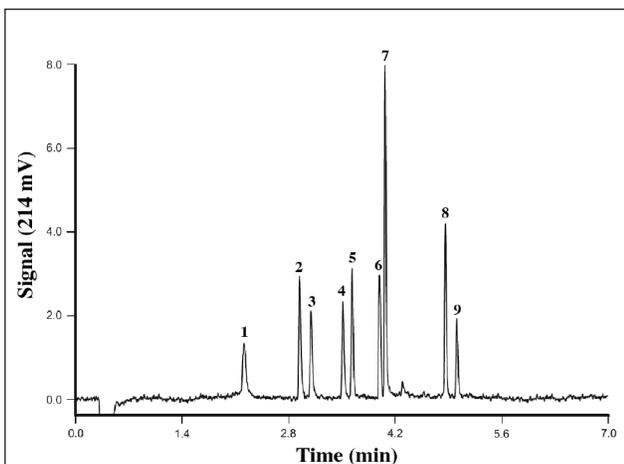
**Figure 3.** Separation of a mixture containing 9 peptides on a monolithic MST–BVPE capillary column (50 × 0.20 mm i.d.). Chromatographic conditions: mobile phase A, 0.1% TFA; B, 0.1% TFA in ACN; 0–30% B in 10 min, 4.0 μL/min, UV 214 nm; injection, 500 nL, 1 ng each. Peaks: bradykinin fragment 1–5, 1; vasopressin [arg8], 2; methionine enkephalin, 3; leucine enkephalin, 4; oxytocin, 5; bradykinin, 6; LHRH, 7; bombesin, 8; and substance P, 9. Reproduced from Reference 53 with permission.
